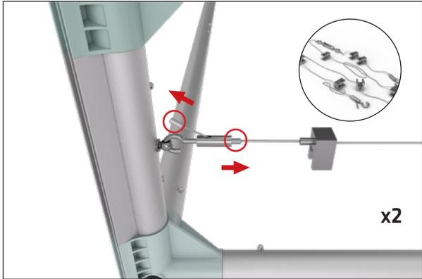
**Step 5:** Move to the center of cable and hand tighten remaining turn buckle to remove any remaining slack. Do not over tighten.
