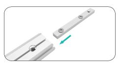
**a.** Remove the screw and insert split connector into one end of the extrusion. Match like colored numbers together. (e.g. 3-3, 4-4).
