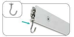
**a.** Eye Hooks: Insert light hooks into the groove in one end of the extrusion.
