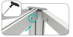
**a.** Place extrusion with the light hooks on top of the extrusion and connect together.
